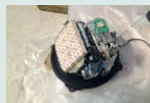
Figure: Ovzon modified on-the-move systems that during testing showed multi Mbps capability on a moving satellite.
