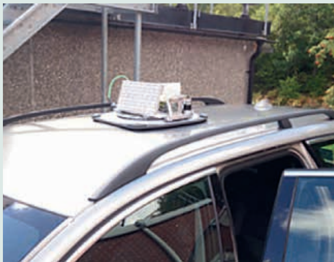
Figure: Ovzon modified on-the-move systems that during testing showed multi Mbps capability on a moving satellite.
