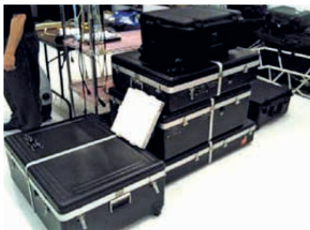
Figure. The photo from 2010 shows the complete Ovzon prototype flat panel terminal (white) on top of one the customer's existing terminal consisting of eight flight cases.
